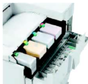
Color and black toner cartridges quickly snap into place, simplifying routine maintenance.
